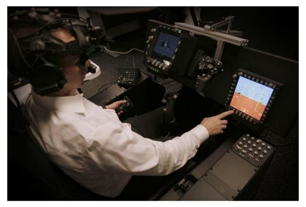
Image: The RVCT Apache cockpit showing MetaVR VRSG view on left hand side sensor (ZedaSoft image).
