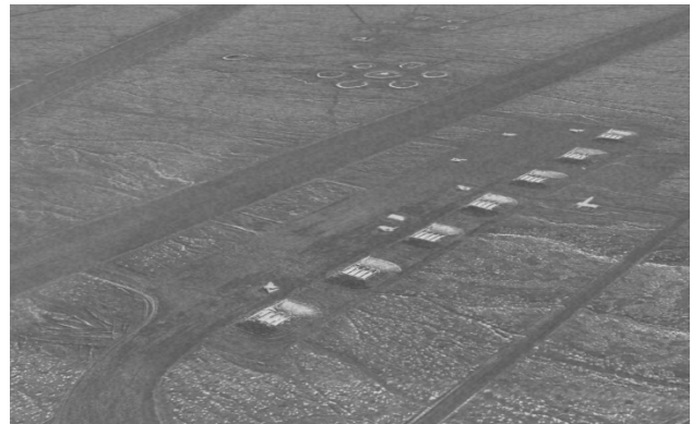
VRSG screen capture of the 2 cm 3D terrain on the left in sensor view. The higher the resolution of the visual database, the more accurate the IR profile for sensor simulation.
