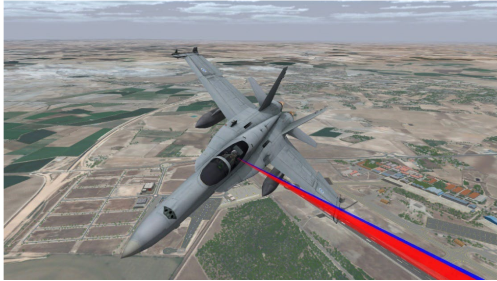
VRSG real-time stealth view of a simulated air mission, rendering the eye-tracking data (head position and pupil gaze) from the pilot trainee wearing a Varjo headset.
