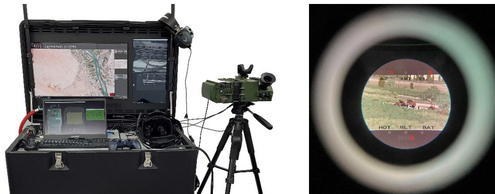
On the left is the Observer station from of MVRsimulation's Deployable Joint Fires Trainer with an emulated SOFLAM to the right mounted to a free-standing tripod. On the right is a view through the lens of the emulated SOFLAM.
