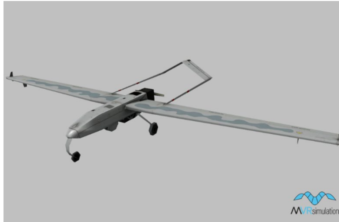
RQ-7B-IE.US model with 302 triangles at the lowest level of detail used to view the model from a distance of 10,000 kms and beyond.
