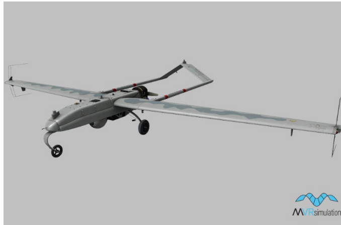
RQ-7B-IE.US model with 45,643 triangles at the highest level of detail used to view the model from a distance up to 2 kms.
