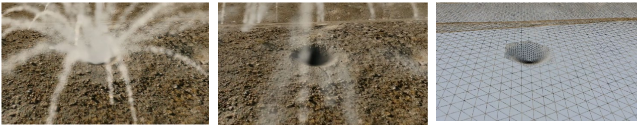
Real-time VRSG screen capture of textured and wireframe views of craters and a crater particle effect triggered by a detonation event rendered on 2 cm per-pixel resolution virtual terrain of the Prospect Square area at the U.S. Army Yuma Proving Ground, AZ. The terrain was built with 2 cm imagery collected by MVRsimulation's data collection small UAV.
