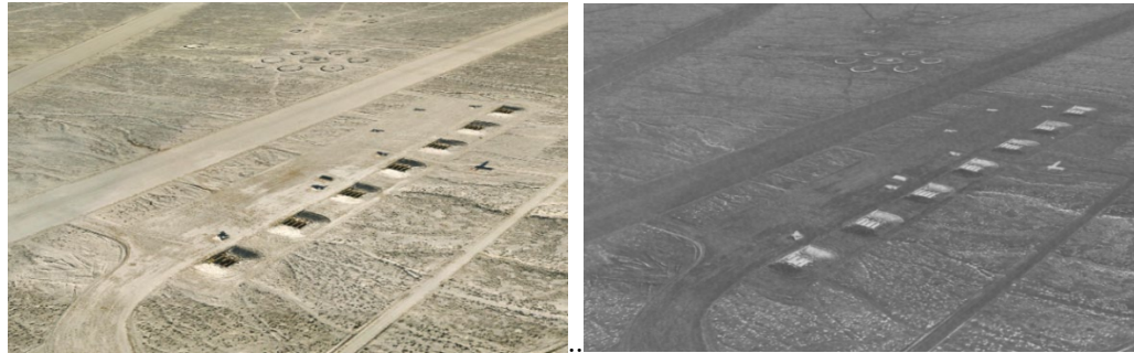
Real-time VRSG rendering of 2 cm terrain built with imagery collected by MVRsimulation's SUAS of the Naval Air Station Fallon Range Training Complex. On the left: visual view, on the right: the sensor view.
