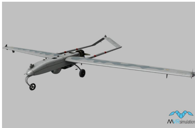
RQ-7B-IE.US model with 6881 triangles at an intermediate level of detail used to view the model from a distance of 300 km.
