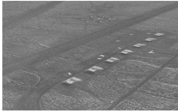
Real-time VRSG rendering in sensor view of the 2 cm terrain shown on the left. The higher the resolution of the visual database, the more accurate the IR profile for sensor simulation.
