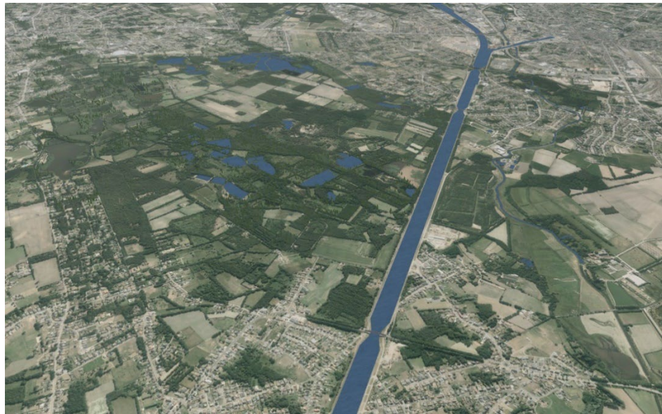
VRSG screenshot demonstrating lakes and rivers. These water features were compiled into the terrain using z-enabled polygons with z-values and the MVRsimulation Legacy Water feature.
