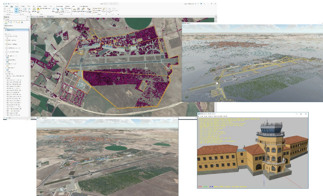
MVRsimulation's Terrain Tools and Virtual Reality Scene Generator (VRSG) real-time textured and wireframe 3D views of the virtual Albacete Air Base, Spain. Also shown is the air base's control tower model in MVRsimulation's Model Viewer.
