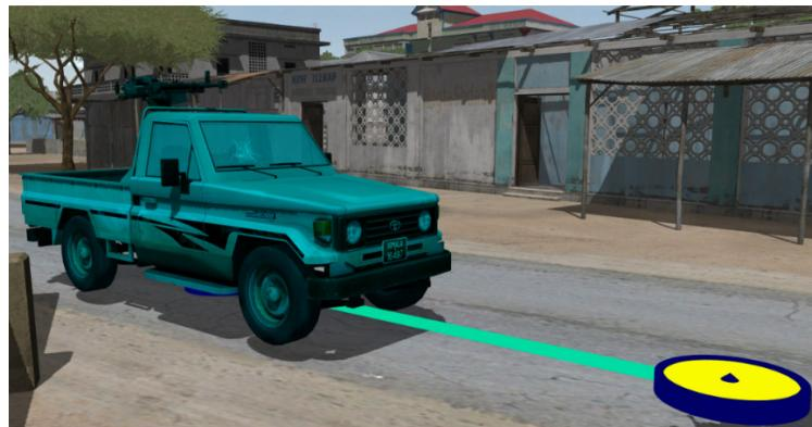
4. Next, click and drag a character model from the behavior feature palette to the scene and drop it onto the vehicle. (In the feature palette, type the search term "human" or just "hum" in the search area to locate the model easily.) When you drop the character on the vehicle, the character automatically assumes the driver position inside the vehicle.
