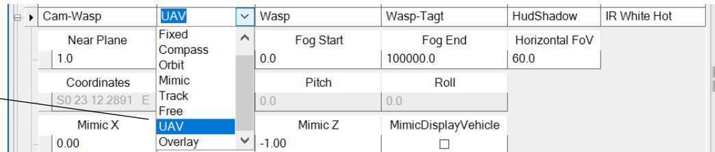
Some attachment modes have their own specific attributes. For example, the UAV attachment mode enables a UAV HUD type to be set, as shown in this next example.
