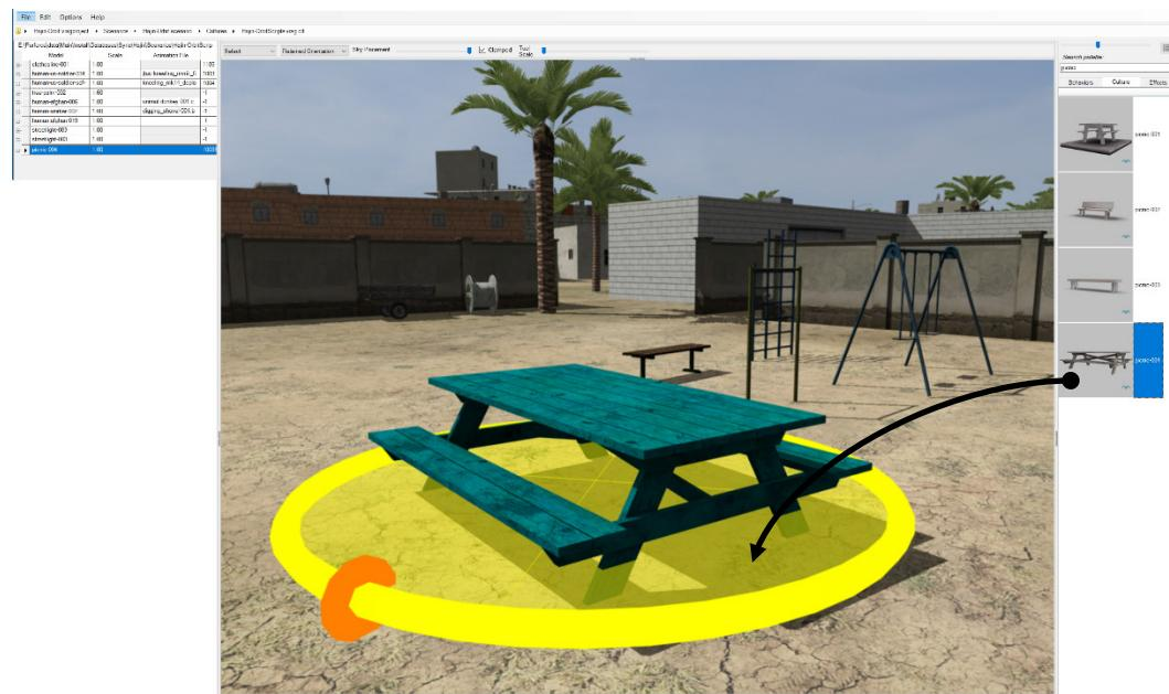
An instance of the model, called an *entity*, appears on the 3D scene where you dragged it. In the example above, a static cultural entity was created on the scene, by dragging a picnic table model from the culture model palette and dropping onto the 3D scene. The new picnic table entity is surrounded by a yellow hoop called the *orientation tool*. Press the Esc key to unselect the entity.
