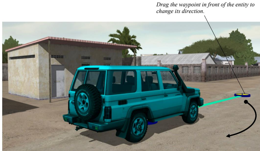
The color of the path ribbon indicates the general speed of an entity's movement along a section of its path. It remains a steady color while the entity moves at a steady speed. The path ribbon color changes from blue at the slowest speed (2.5mph or below), through green to yellow at the maximum speed. For human character entities, the path ribbon is yellow at speeds of 7m/s (15.5mph), and for vehicle entities at speeds of 20m/s (45mph) or faster.
