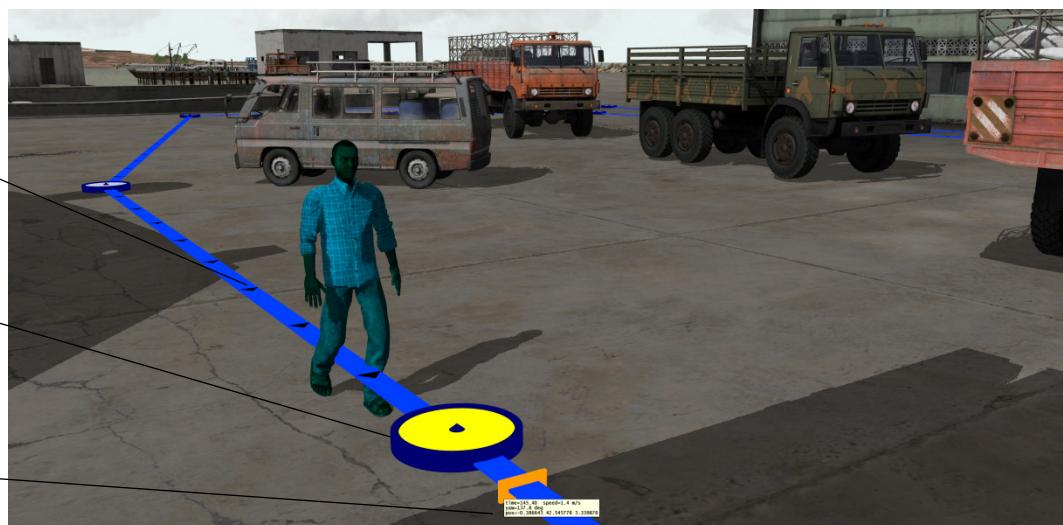
In Scenario Editor, you can change the model assigned to a behavior entity. In the behavior table, click in the cell for the model assigned to the entity to choose a different model of the same type (culture or behavior) and same DIS Kind and Domain from the drop-down menu. A change in the model does not change the marking (the entity/instance name).
