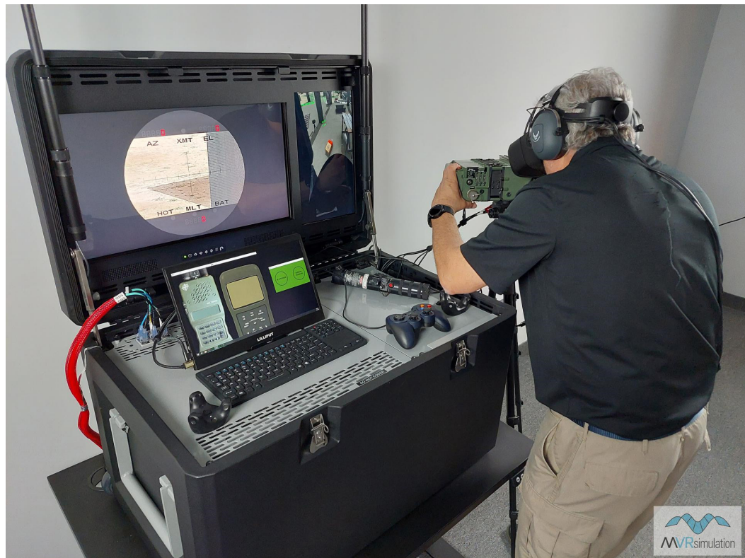
MVRsimulation's DJFT Observer Station trainee looking through the Varjo XR-3 headset at the VRSG scene displayed in the emulated SOFLAM. The main screen shows the view inside the emulated SOFLAM.
