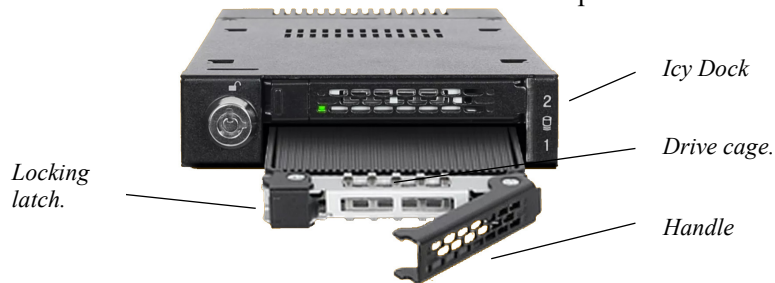
Hard drive cage being installed into the Icy Dock.
