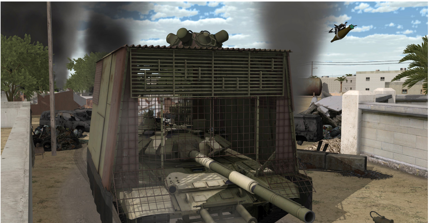
Real-time VRSG scene in the devastated urban terrain of Hajin, Syria with the new 3D model of a Russian T-72B3 Turtle Tank. This model of the T-72B3 includes an integrated drone cage with mine plow roller. Attacking in the image is a first person view (FPV) UAV racer-style drone with RPG-7 warhead.
