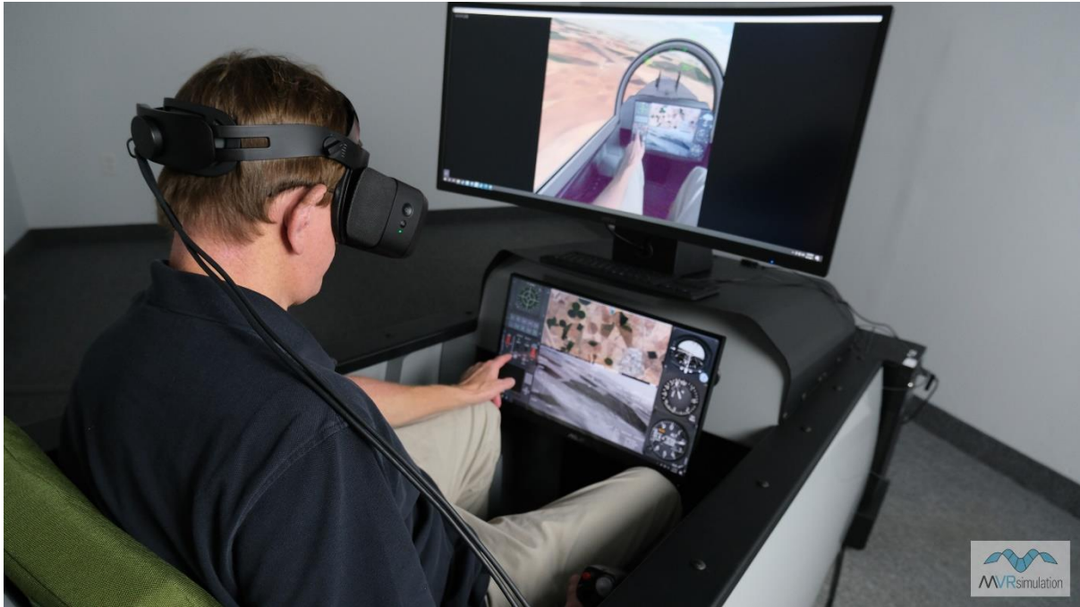
Image: Flying in MVRsimulation's Part Task Mission Trainer (PTMT) wearing the Varjo XR-3 mixed reality headset. VRSG renders the out-the-window view in the headset and on the curved display. (Notice the pilot's hand on the controls is visible in the VRSG view.)
